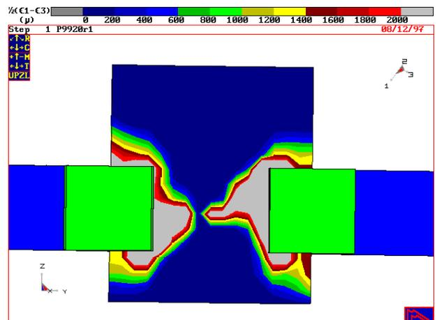
Substantial yield has occurred in the walls, and slowly extending to the pillar core. At the next step the core fails in shear.
