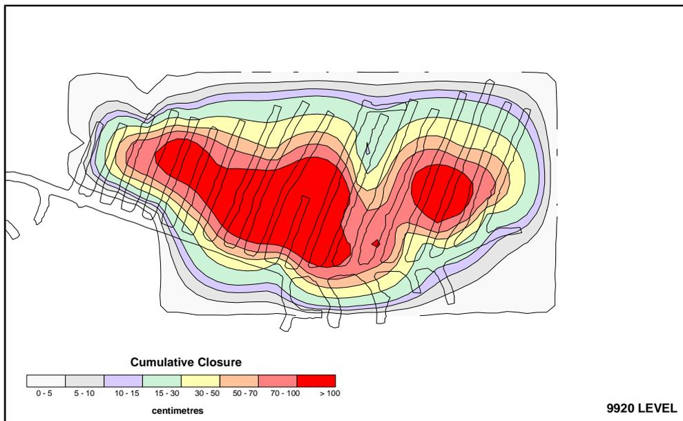
Figure 12 - Convergence monitoring data for 9,900m Level to April 1999
