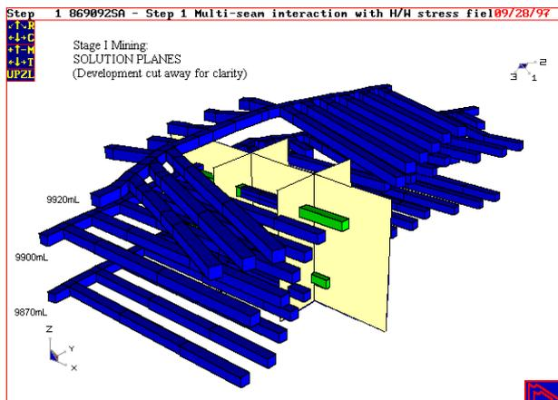
Figure 7 - Material zones around cross-cuts
